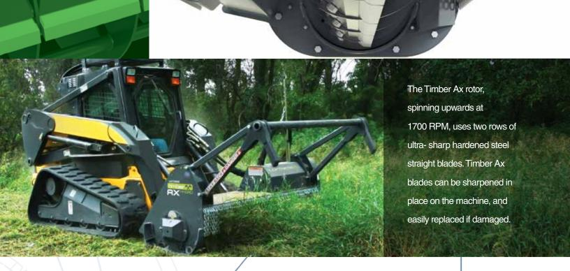
The rotor is designed for extreme conditions and can withstand intense use. Unique to the Timber Ax is the reverse, upward rotation of the rotor and blades. As material is engaged, it is directed up off the ground and positioned against the adjustable recutter bar. Keeping the cutting action away from the ground helps maintain rotor energy, reduces knife wear, and processes brush, branches and trees into a consistent particle size.
