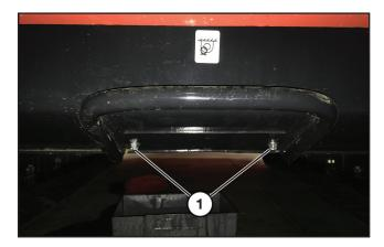
Remove the two bolts (1) securing the cover to the bottom of the track loader and lower the cover.
