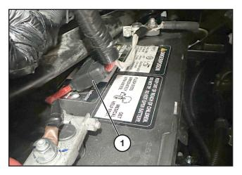
Connect the fuse holder (1) (supplied with the oil cooler) to the red (8 AGW) wire from the cooler harness, and to the battery positive.
