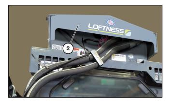
Place the rear cover (2) back onto the Loftness oil cooler. Reinstall all hardware and tighten.
