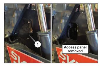
Remove the screened access panel (1) on the rear left side of the loader and set aside.
