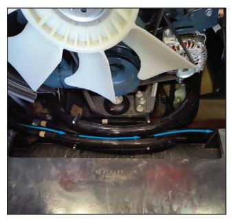
Continue routing the harness along the back of the engine bay toward the battery.
