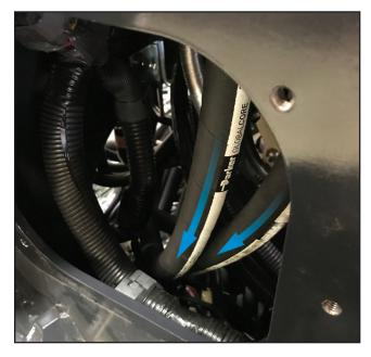
Route both hoses, one at a time, down into the engine bay as shown. Use the opening from the screened access panel that was removed earlier to assist with routing.
