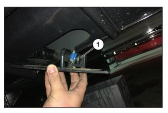
Remove the drain plug (1) and drain the hydraulic oil.
