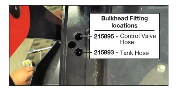
Install the bulkhead fitting with control valve hose (215895) into the front hole (closest to the cab) and secure with the nut.
