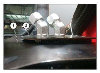
Temporarily set the cover panel (1) - part no. 212507 into position and check to make sure the bulkhead plate (2) is level with the cover panel.
