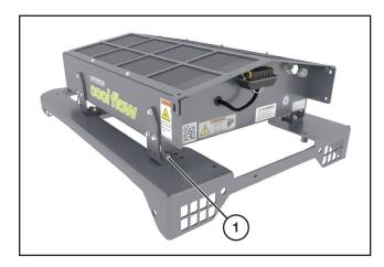
Using a hoist, lift the oil cooler and place on top of the cooler mounting frame. Align the slotted holes in the mounting brackets to the holes in the mounting frame.
