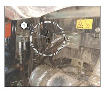
Locate the metal line (1) under the cab.
