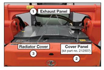
Reinstall the exhaust panel (1) first. Then install the cover panel (2) - part no. 212507 from the Loftness cooler kit. The radiator cover (3) is reinstalled last.
