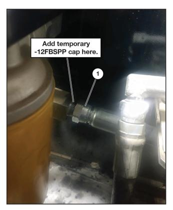
NOTE: Take note of the path/route of the Kubota factory hose and where it is secured. The new cooler kit hose will be installed in its place and will follow the same path.
