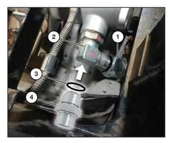
Disconnect the factory line (1) from the cooler core and remove the elbow (2).
