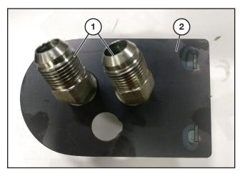
Install the two bulkhead fittings (1) - part no. 202975 at  $45^{\circ}$  onto the bulkhead plate (2) - part no. 212506 as shown.
