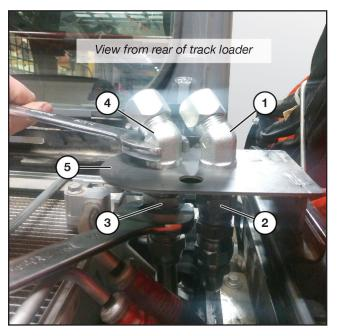
Connect the core assembly line (1) to the outside 45° bulkhead fitting (2), then connect the tank line union (3) to inside 45° bulkhead fitting (4)
