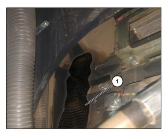
Route the new hydraulic hose (1) - part no. 212697 using the same path as the Kubota hose and steel line that was just removed.
