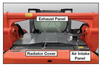
The panels and covers called out above will need to be removed from the track loader to begin the installation. Refer to your Kubota SVL75-3 owner's manual for removal instructions.
