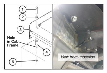
When the front holes are aligned, insert a bolt (1) - part no. 4496 with washer (2) - part no. 4068 from the top side of the cooler mount (3), and install a spacer (4) - part number 212428 on the underside of the cooler mount.
