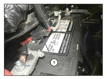
Connect the fuse holder (supplied with the oil cooler) to the red (8 AGW) wire from the cooler harness, and to the battery positive.
