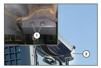
Remove the two inner bolts (1) securing the front left side headlight (2).
