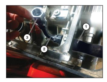
Connect the upper end of the hydraulic hose (1) to the elbow tube (2) - part no. N28906 with adapter fitting (3) - part no. N28841 from the cooler kit. Tighten in the vertical orientation as shown.
