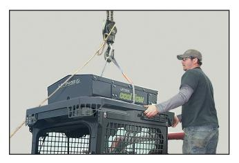
Lift the cooler kit and place into position on top of the track loader cab.
