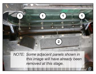
Remove the four bolts with washers (1) by the rear window and remove the panel (2).
