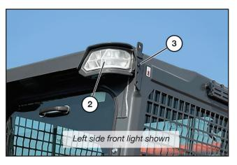
While supporting the light (2), remove the outer bolt (3).
