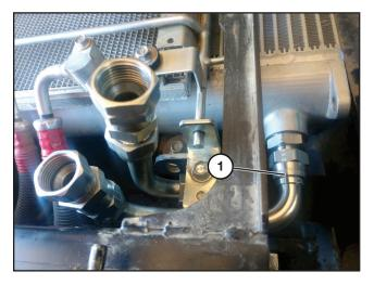
Remove the temporary cap on the core fitting and install the tube assembly (1) as shown. Do not tighten the fittings yet.
