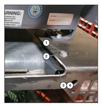
When the holes adjacent to the rear cab lights are aligned, insert a bolt (1) - part no. 4218 with washer (2) - part no. 4068 from the top side of the cooler mounting frame as shown above.
