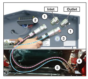
Connect the two elbow fittings (1) - part no. N19270 to the oil cooler INLET and OUTLET ports and position at the angle shown above.
