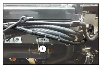
Continue routing the cooler harness (1) below the factory track loader's harnesses and to the left side of the track loader as shown.
