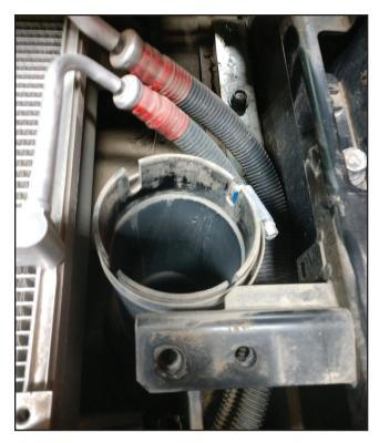
Remove the air intake and the bracket as shown above. Refer to your Kubota SVL75-3 owner's manual for instructions.
