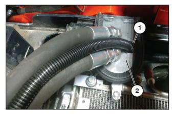
Route the cooler harness alongside the cooler hoses and through the bulkhead plate. Make sure to provide enough slack in the harness to avoid binding and pinch points when tilting the cab.
