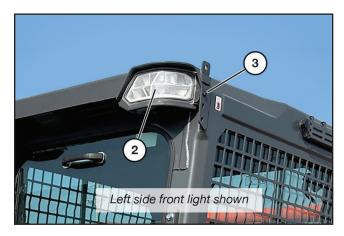
While supporting the light (2), remove the outer bolt (3).
