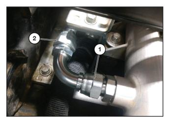
When level, tighten the core swivel fitting (1) first, then tighten the tube assembly swivel fitting (2).
