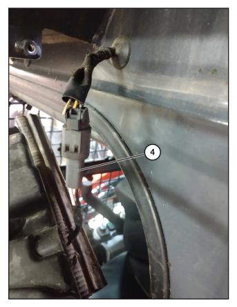
Disconnect the headlight wiring harness (4) and carefully remove the light. Set aside.
