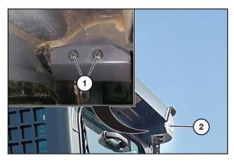
Remove the two inner bolts (1) securing the front left side headlight (2).
