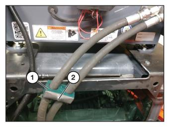
Install the hose clamp (1) - part no. N29662 and route hoes as shown above. Install the clamp bolt (2) - part no. 4004. Do not tighten at this time.
