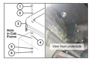
When the front holes are aligned, insert a bolt (1) - part no. 4016 with washer (2) - part no. 4068 from the top side of the cooler mount (3), and install a spacer (4) - part number 212428 on the underside of the cooler mount. From the underside of the cab frame, install a washer (5) - part no. 4068 and nut (6) - part no. 4054 onto the bolt. Hand tighten the hardware.
