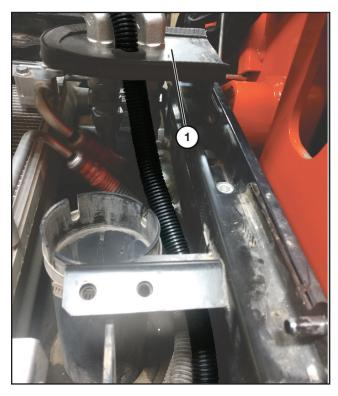
From the bulkhead plate (1), route the cooler harness alongside the track loader harnesses adjacent to the air intake as shown.
