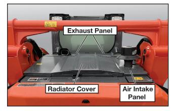
The panels and covers called out above will need to be removed from the track loader to begin the installation. Refer to your Kubota SVL75-3 owner's manual for removal instructions.
