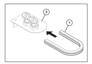
Install the seal trim (1) - part no. 212573 onto the bulkhead plate (2).
