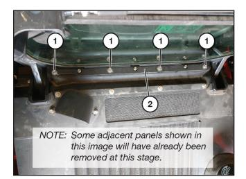
Remove the four bolts with washers (1) by the rear window and remove the panel (2).
