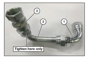
On a work bench, lay out and assemble the short elbow tube (1) - part no. N28902, long elbow tube (2) - part no. N28906, and union fitting (3) - part no. N25884.
