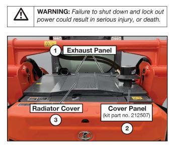
Reinstall the exhaust panel (1) first. Then install the cover panel (2) - part no. 212507 from the Loftness cooler kit. The radiator cover (3) is reinstalled last.
