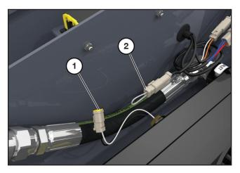
Remove the temperature sensor plug (1) on the main harness.
