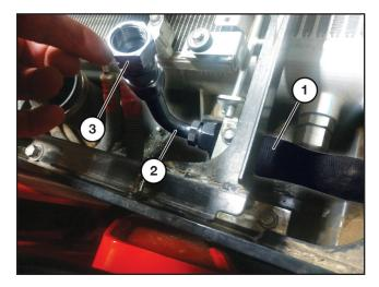
Connect the upper end of the hydraulic hose (1) to the elbow tube (2) - part no. N28906 with adapter fitting (3) - part no. N28841 from the cooler kit. Tighten in the vertical orientation as shown.
