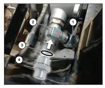
Disconnect the factory line (1) from the cooler core and remove the elbow (2).
