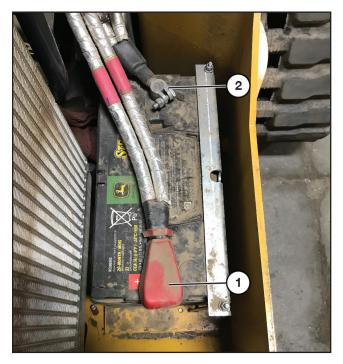
Connect the fuse holder (supplied with the oil cooler) to the red (8 AGW) wire from the cooler harness, and to the battery positive (1).
