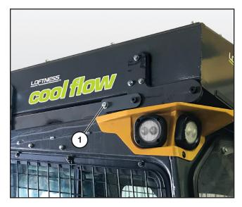
Remove the hex bolt (1) securing the lifting leg in the storage position. Repeat this process for the corresponding bolt on the lifting leg on the opposite side.
