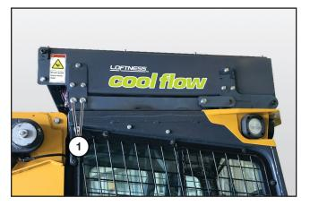
Remove the two bolts (1) securing the rear legs to the mount. Repeat this process for the corresponding bolts on the rear legs on the opposite side.
