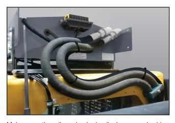
Make sure the oil cooler hydraulic hoses and wiring harness are secure. The hydraulic hoses and wiring harness coming from the oil cooler should route as shown above.
