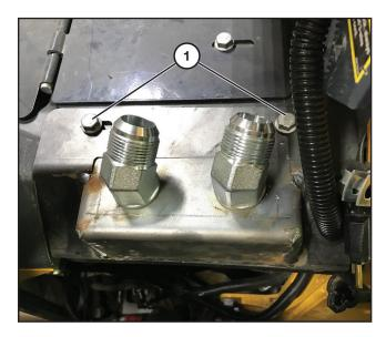
Using the two bolts (1) that were removed from the small panel, secure the bulkhead panel assembly onto the frame in the same location as the former panel.
