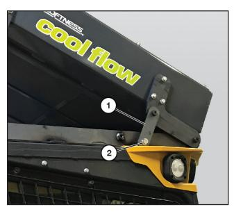
Using a hoist, lift the rear of the oil cooler up and pivot the lifting legs (1) (both sides) until the open holes in the legs align with service position holes in the cab mount. Reinstall the bolts (2) (both sides).
