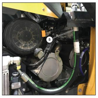
Connect the other end of the hose to the rear bulkhead fitting (5). Tighten.
