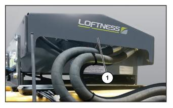
Reinstall the back access cover (1) onto the oil cooler and tighten the bolts.
