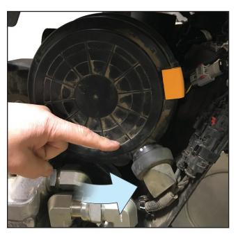
Turn the air filter cover so the drain is positioned as shown above.
