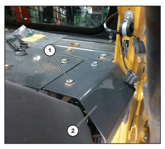
Unscrew the two bolts (1) and set aside. These bolts will be used to secure the new bulkhead.
