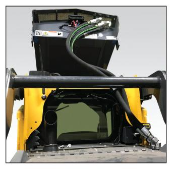
Make sure the hydraulic hoses are routed as shown above and all hose and fitting connections are tightened.
