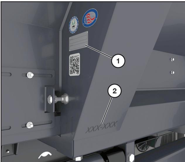
The machine serial number is shown in the tag (1) located at the front of the hopper, left side; and is also stamped into the hopper frame (2) near the tag.
