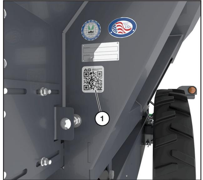
To access a digital parts book and/or owner's manual, use a smart phone to scan the QR Code (1) located just above the serial number tag on the front of the hopper. This code will provide a link to machine documentation on the Loftness website.
