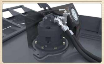
**Radial Piston Motor**: A 150cc radial piston motor provides instant torque at start-up for fast recovery times. It requires 28-45 GPM up to 5000 PSI and 50-110 hydraulic horsepower.
