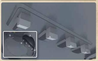
**Carbide Teeth**: The Kwik Cut comes standard with 18 carbide teeth mounted on the underside of the disc. They are designed to grind stumps and brush to the ground. The teeth are mounted to the disc with a single bolt, so they can be easily replaced on the jobsite using a common hex socket.
