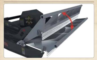
**Floating Door:** A hinged door at the front of the brush cutter opens when pushed against a tree to expose the blades. When fully opened, the door becomes solid, acting as a tree pusher.
