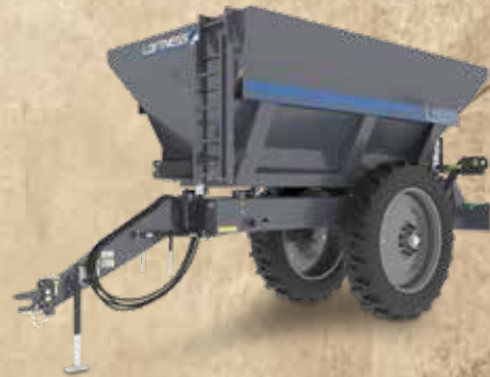
L1230 // 12-Ton Lime/Fertilizer Spreader
