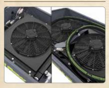
High Capacity Cooling: The single-fan model offers an impressive 95,000 BTUs per hour of cooling capacity for mid-frame skid steers. The twin-fan Cool Flow offers industry-leading cooling performance for extreme temperatures and job applications with 150,000 BTUs per hour.
