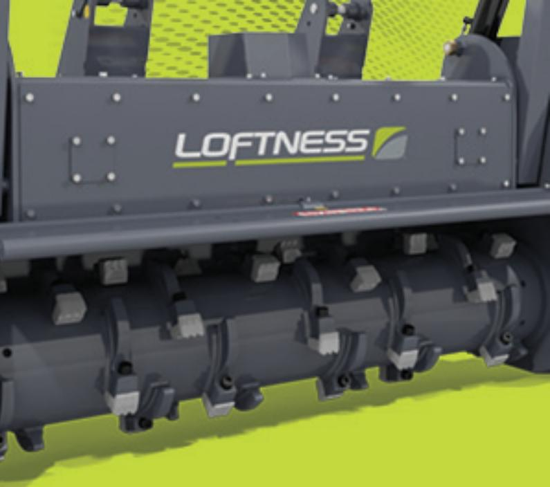
» **A staggered tooth arrangement** ensures single-tooth contact with the work surface at all times while maintaining optimal rotor balance.
