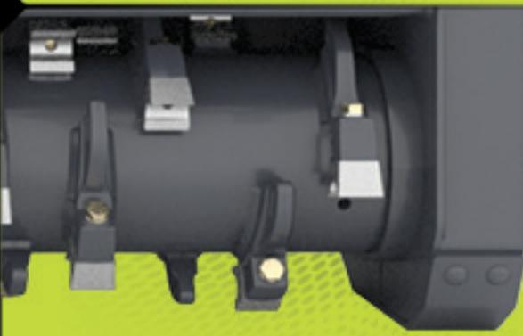
» **The Battle Ax has specialized anti-wrap protection** to help prevent debris from entering the bearing chamber.
