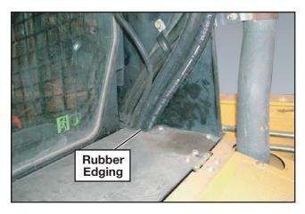
You may need to cut holes in the engine hood or sheet metal as the hoses pass from under the hood up towards the Loftness Universal Oil Cooler. Line the newly cut sheet metal edge with rubber edging.
