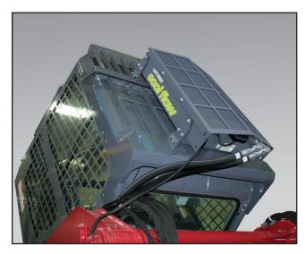
Raise cab and check that the hoses from the roof cooler do not pinch against the cab or hood structure.
