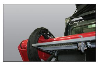
Route the hoses along one side. Make sure the hoses will not be pinched or kinked. Also make sure the hoses will not rub on sharp edges, hit moving parts (fan, belts), or rest against hot surfaces (exhaust, muffler, etc).
