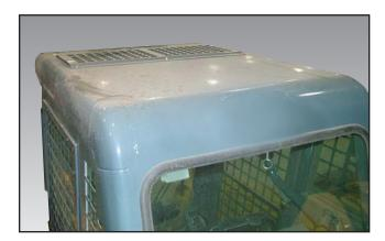
The first step is to determine the best location to physically mount the oil cooler. The cleanest, coolest air available will deliver the best oil cooling results. The oil cooler draws air in from the bottom and blows it out the top.
