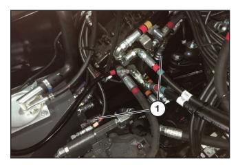
Remove return hose (1) at each end shown above. This hose will no longer be used. Hoses for the oil cooler cab mount kit will be connected in these two locations.
