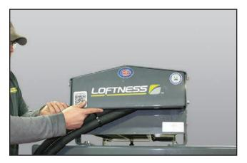
Place rear cover back onto the oil cooler. Reinstall bolts (4 total) and tighten.
