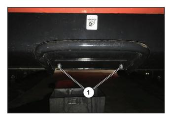
Remove the two bolts (1) securing the cover to the bottom of the track loader and lower the cover.
