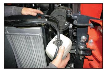
Detach coolant overflow tank to access battery terminals.
