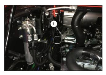
Inside the engine compartment, add the hose brace (1) that is supplied with kit. This brace will support the cooler hoses that will be added and prevent them from coming in contact with track loader engine components.
