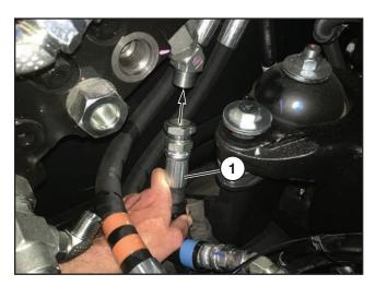
Connect the other end of the INLET hose (1) to the fitting on the control valve as shown above. Refer to drawing on page 4 for an illustrated schematic.
