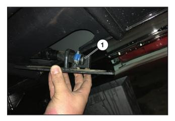
Remove the drain plug (1) and drain the hydraulic oil.
