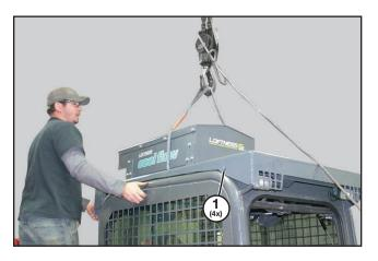
Lift the oil cooler with frame and place into position on top of the track loader cab.
