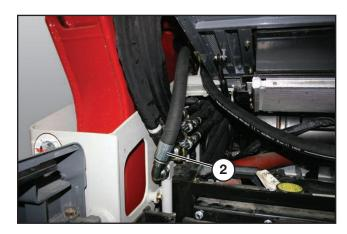
Connect the opposite end of the short hose to the manifold on track loader. Tighten.
