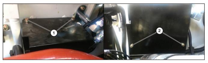
Remove the four bolts and cover to gain access. Use a 13 mm wrench to remove the top bolts (1) and a 10 mm wrench to remove the lower bolts (2).
