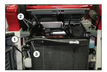
Replace hose guide (1). The two oil cooler hoses (2) should be routed through the guide as shown.
