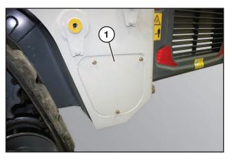
Unfasten the three bolts and remove the battery access panel (1).
