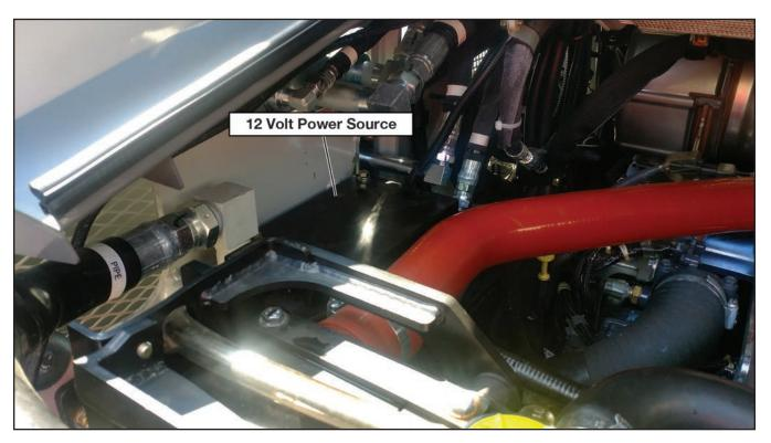
The 12 volt power source is accessed via the left side of the rear engine compartment.
