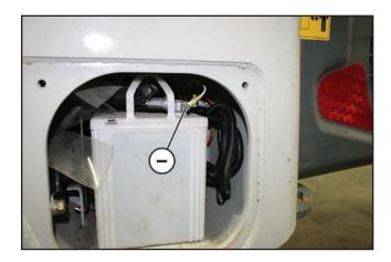
Connect the white negative (-) 8 AWG and 18 AWG wire of the oil cooler harness to the negative terminal on the battery.
