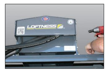
Remove the shipping tie-wraps securing the wiring harness to the cooler and put the rear cover back and oil cooler. Tighten the hardware.
