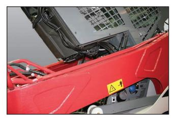
Tilt the cab up on the track loader to provide access to the wiring harness located underneath the cab.
