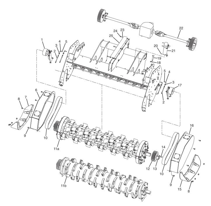
Note: Both Rotor selections are shown. Item 11a Rotor is equipped with Hammers. Item 11b Rotor can be equipped with either Double Carbide, Planer Carbide, or Quadco Planer teeth. See parts list on page 36 & page 37 for rotor part number variations.
