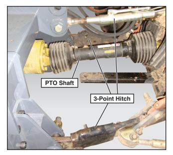
Attach the tree hammer to the tractor using the 3-point hitch.
