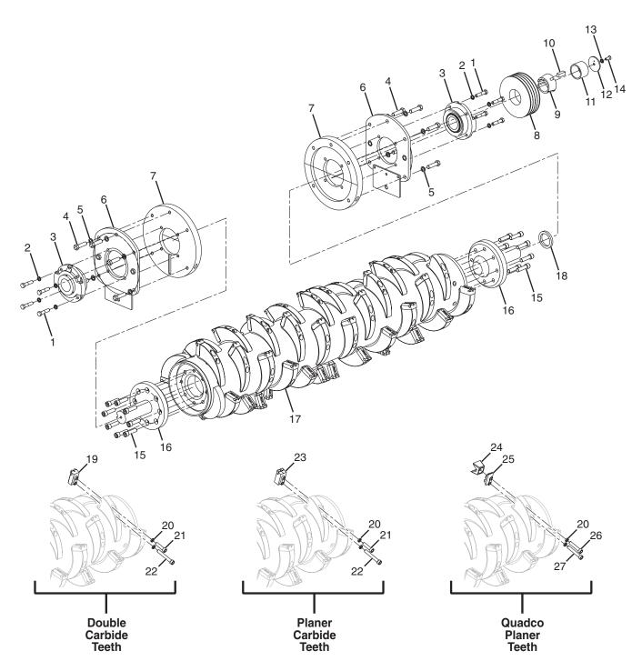
To order complete Rotor with Double Carbide Teeth, use part number N28400. To order complete Rotor with Planer Carbide Teeth, use part number N28678. To order complete Rotor with Quadco Planer Teeth, use part number N28679.
