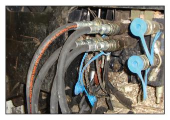
If equipped with hydraulic door and/or hydraulic pusher bar operation, install the hydraulic quick couplers to the hydraulics on the tractor.
