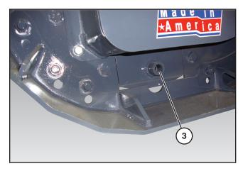
Remove the rotor lock pin from the storage compartment and insert into the locking hole (3) on either the left or right side of the unit.
