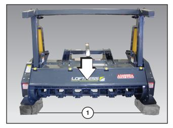
Raise the tree hammer off the ground and place blocks (1) underneath the skids. Lower the tree hammer down on the blocks.
