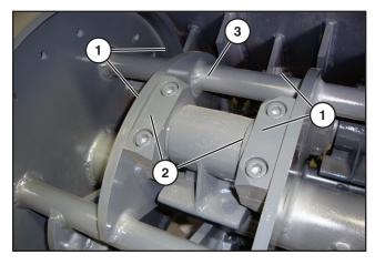
Remove the four bolts (1) and pull out the two mounts (2), the hammer (3), shaft, and washers.
