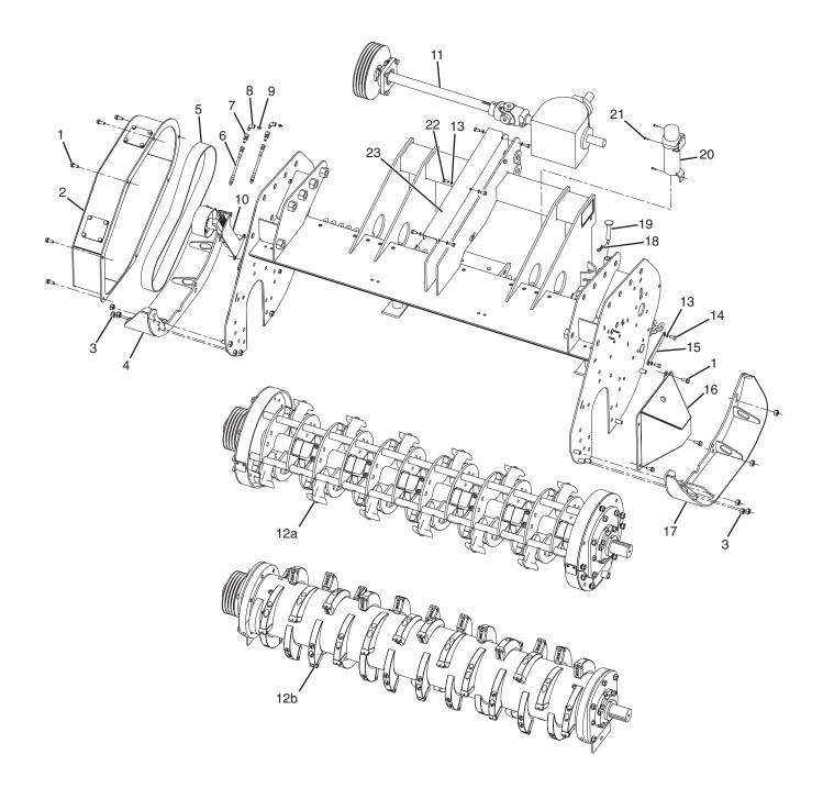
Note: Both Rotor selections are shown. Item 12a Rotor is equipped with Hammers. Item 12b Rotor can be equipped with either Double Carbide, Planer Carbide, or Quadco Planer teeth. See parts list on page 36 & page 37 for rotor part number variations.
