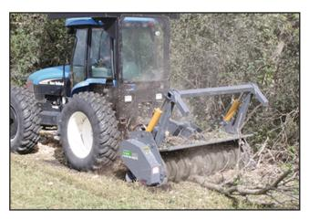
Maintain a constant work height by carrying the weight of the tree hammer on the 3-point hitch. Skid shoes should only be used to prevent scalping on uneven ground. Minimizing the vertical movement of the 3-point hitch will greatly improve the life of your PTO.
