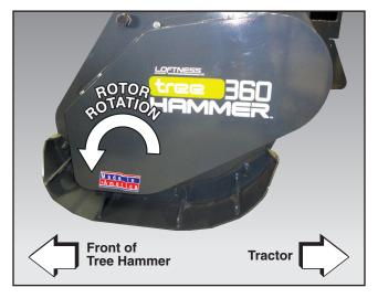
Engage the tractor PTO, the rotor should start rotating in a forward direction. The rotation should be counterclockwise as viewed from the right side of the tree hammer.
