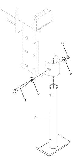
Note: The Tree Hammer is equipped with two Jack Stands. Only one is shown for parts listing.
