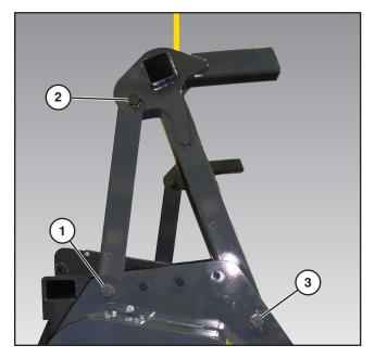
Remove bolt (1) from the lower storage position. Loosen the two bolts (2 & 3) to allow the pusher bar to pivot forward. This must be done on both sides.
