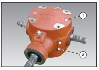
Remove the plug from the upper port (1), and the plug from the lower port (2).
