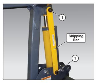
To remove the shipping bar, unfasten the two 1-1/4" nuts (1) and take out the shipping bar. Return the two nuts to their original position and tighten.
