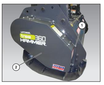
Remove the seven bolts (1) and drive belt cover (2).
