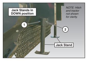
Once securely attached to the 3-point hitch of the tractor, the jack stand position can be adjusted.
