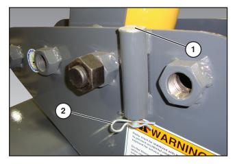
The rotor lock pin (1) with clip (2) is stored on the frame inside the right side pusher cylinder. Use the rotor lock pin to keep the rotor from spinning when performing any work or maintenance on the rotor or hammers, or when transporting the tree hammer.
