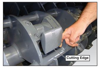
To install a new hammer, reverse the order of the removal procedure. Make sure that the cutting edge of the hammer is pointing down. See the photo above for hammer orientation.
