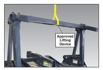
**NOTE:** Adjusting the pusher bar requires two people or the use of an approved lifting device to support the push bar as it is being adjusted.
