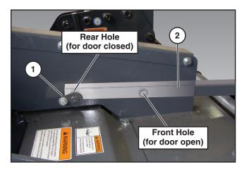
Remove the bolt, washer, and pin (1).
