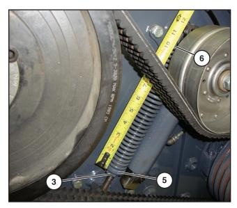
Turn the adjustment bolt clockwise until the distance from the collar (5) to the end of the spring (6) is approximately 10-1/4". Tighten jam nut (3).
