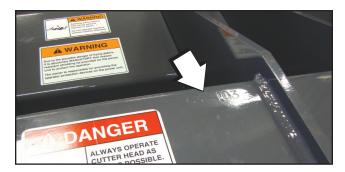
The serial number is also stamped into the frame, on top of the hitch support.
