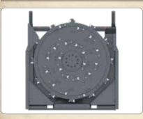
Housing Design: The sides of the Bad Ax housing are parallel. This design provides optimal control when compared with funnel, or V-shaped, disc mulchers, which can be easily misdirected when hooking onto stumps or other solid objects.
