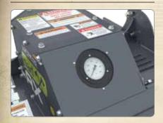
**Instrumentation**: A rubber-mounted pressure gauge allows the operator to easily monitor the workload from the skid steer cab.
