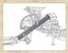
**Transition Auger**: The 13-inch diameter transition auger delivers grain to the pivot point over the base of the main auger.
