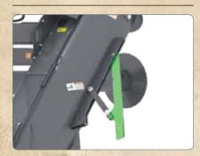
**Bag Knife**: Two cutting positions ensure a positive cut through any bag shape.
