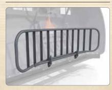
**Bag Cradle**: Combined with the 4,000-pound electric winch, the cradle lifts the bag from ground level into position. It easily folds and stores inside the tunnel after use.
