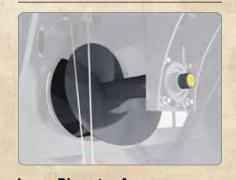
Large Diameter Auger: The 20-inch main discharge auger offers ¼-inch thick abrasive resistant steel flighting for long life.
