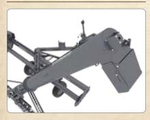
**Main Auger**: The 17-inch main auger made with ¼-inch flighting achieves load transfer rates of 8,500 bushels per hour.
