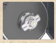
**Bag Removal Clutch**: Operator can simply disengage the roller drive by hand and bag can then be rolled off the bag roller tube.
