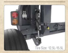
**Axle Lift**: Hydraulically controls the height of the cross augers inside the bag.
