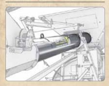
**Main Auger**: The high speed 13-inch diameter main stationary lift auger moves grain into the hopper of the bag loader.
