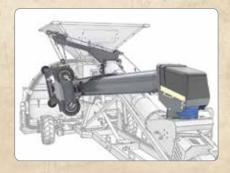
**Hopper Transport**: The swing hopper and auger are easily winched up into transport position with a cable/pulley system.
