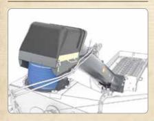
**Swing Auger**: A 13-inch diameter swing auger provides easy reach and positioning control when aligning the hopper under the truck's discharge chute.
