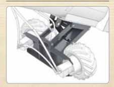
**Hopper Lift**: Used in conjunction with the drive wheels to make simple work of properly positioning the swing hopper.
