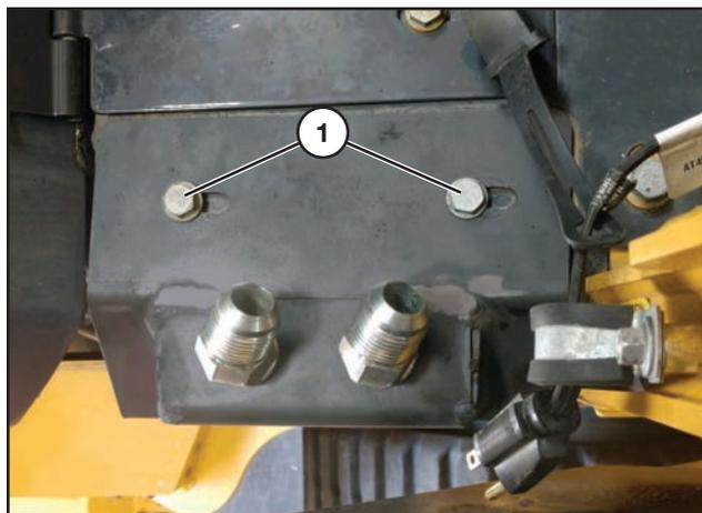
Using the two bolts (1) that were removed from the small panel, secure the bulkhead panel assembly onto the frame in the same location as the former panel.
