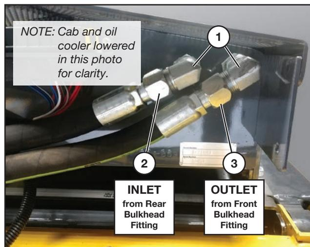
Install the two 90-degree elbow fittings (1) (Loftness part no. N19270 in the cooler hose kit) onto the two straight oil cooler fittings. Secure the fittings at the angles shown above. Tighten both fittings.
