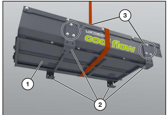
Suspend the universal oil cooler (1) with a hoist and straps.
