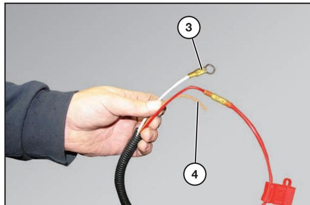
Strip the end of the white negative (-) 18/8 AWG wire and attach a ring terminal (3).
