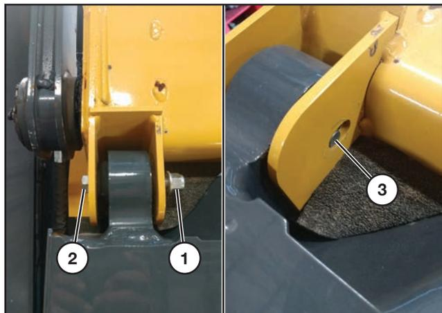
Remove the lock nut (1) on the John Deere cab pivot bolt (2), then back the bolt out so the threaded end is flush with the frame (3).
