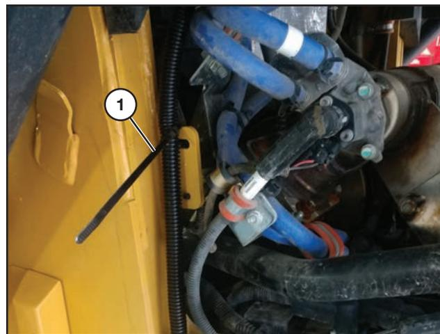
Secure the wiring harness with zip-ties (1) as needed to avoid direct contact with moving parts and/or hot components within the engine bay.
