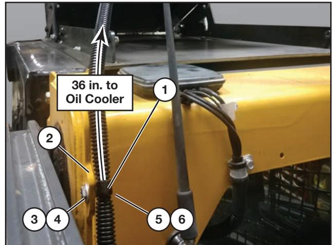
Route the wiring harness from the Loftness oil cooler along the rear left side of the track loader.
