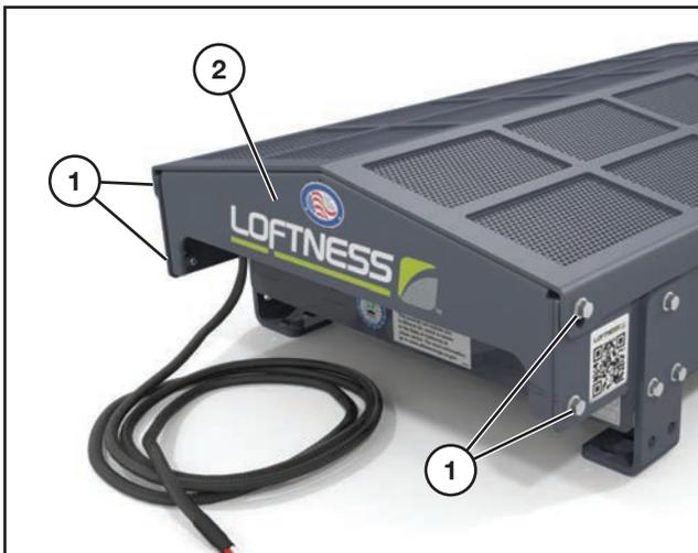
While the oil cooler is still on the ground remove the four bolts (1) securing the back cover (2) to the cooler frame.
