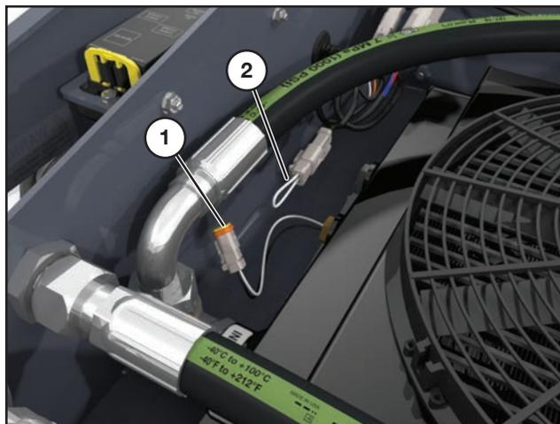
Remove the temperature sensor plug (1) on the main harness.
