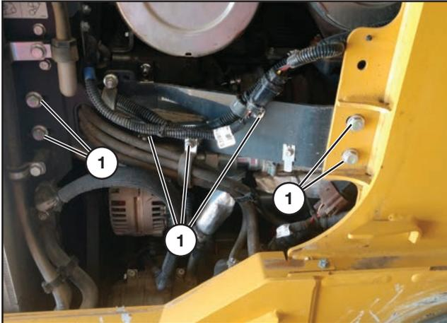
Remove the hardware at the locations shown (1) to gain access to the return line that routes between the factory-installed oil cooler and the hydraulic tank.
