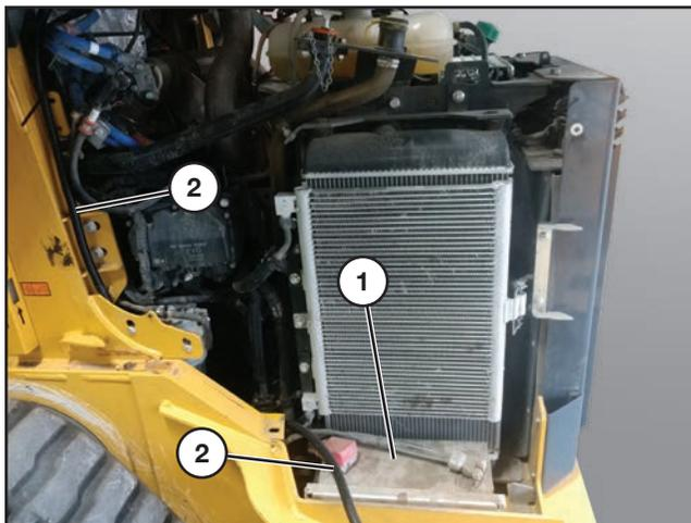
With the left side engine panel removed, locate the battery (1) and make sure it is clear of any debris.
