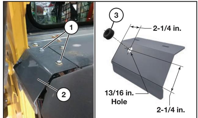
Remove the two bolts (1) and pull out the left side body panel (2) located behind the cab.
