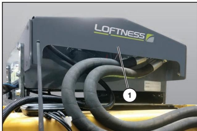
Reinstall the back access cover (1) onto the oil cooler and tighten the bolts.
