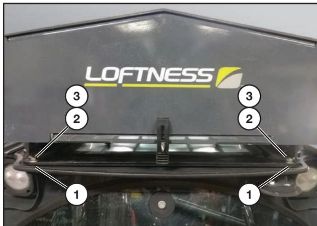
Lower the front of the oil cooler down onto the cab.
