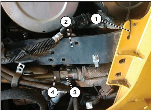
Use a zip-tie (1) to temporarily secure the bracket (2) away from hydraulic line.
