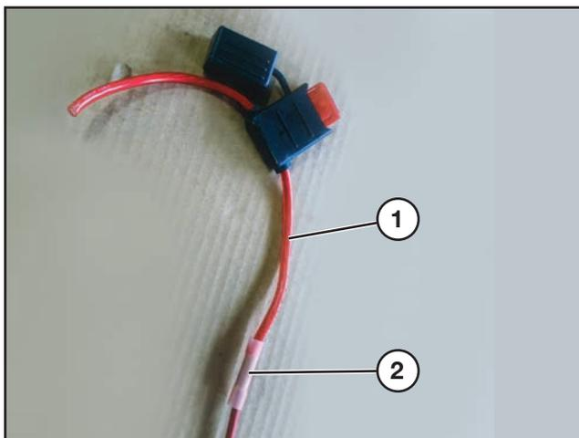
Cut the loop of the inline fuse holder (1) at the half-way mark, keeping an equal length of wire on either side of the fuse holder. Strip both ends of the wire.
