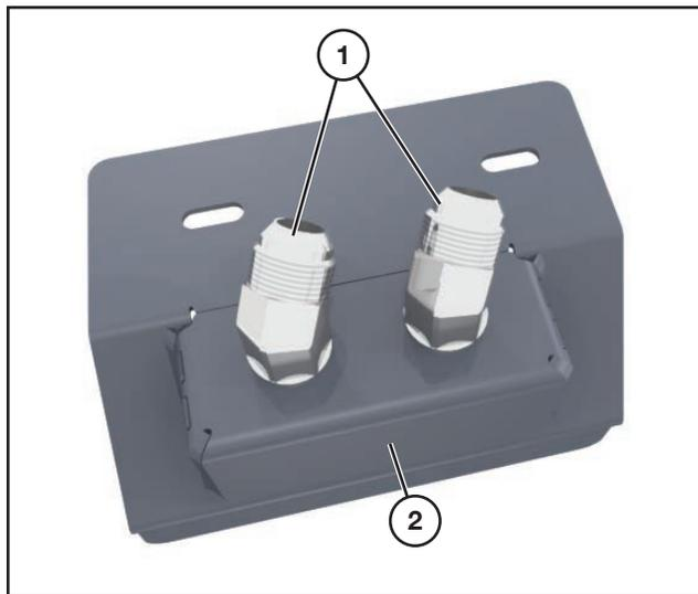
Install the two bulkhead fittings (1) (Loftness part no. 202975 in the cooler hose kit) onto the new bulkhead panel (2) in the direction shown. Tighten the fittings.
