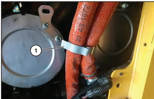
Use the metal tie-band (1) from the kit to secure the two hoses together.
