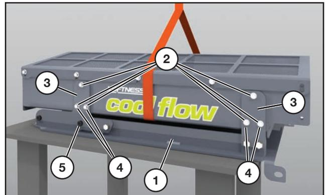
Install the oil cooler onto the cab mount (1).
