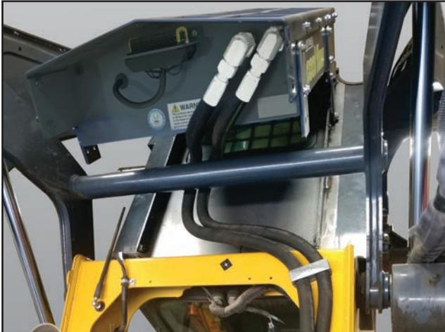
Make sure the hydraulic hoses are routed as shown above. Tighten all connections.
