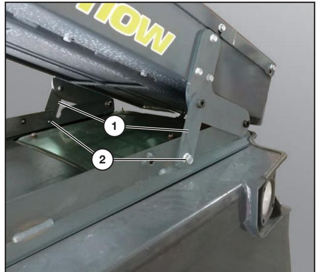
Using a hoist, lift the rear of the oil cooler up and pivot the lifting legs (1) until the open holes in the legs align with service position holes in the cab mount. Reinstall the bolts (2).
