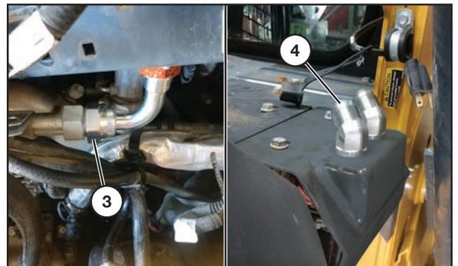
Connect the 90-degree end of the 26 in. hydraulic hose (Loftness part no. 209055 in the cooler hose kit) to the steel cooler line (location 3).
