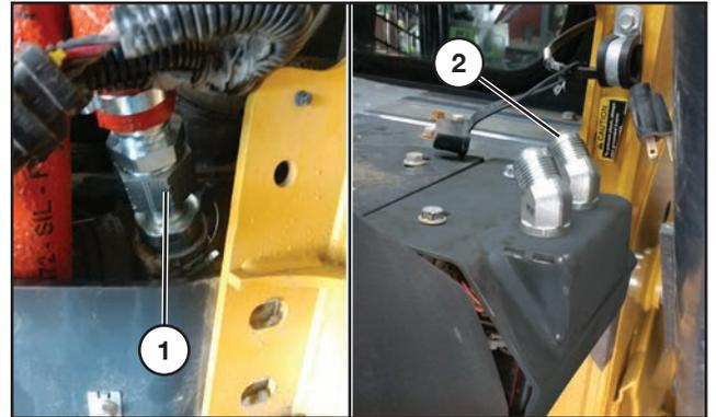
Connect one end of the 19-1/2 in. hydraulic hose (Loftness part no. 209053 in the cooler hose kit) to the flexible tank line (location 1).
