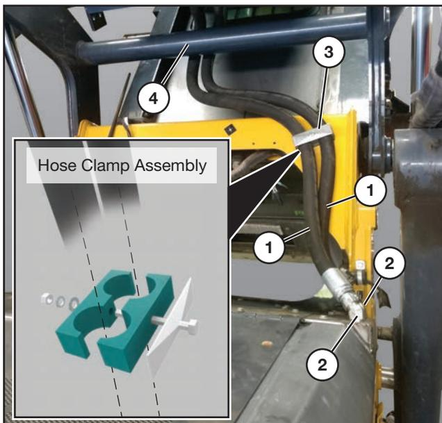
Connect one end of each 63 in. hydraulic hoses (1) (Loftness part no. 209051 in the cooler hose kit) to the bulkhead fittings (2) as shown. Tighten both connections.
