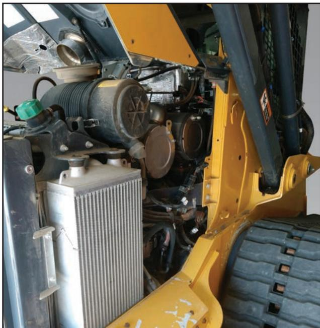
Lift the rear engine compartment door up and remove the right and left side engine panels. Refer to the John Deere track loader owner's manual for instructions.
