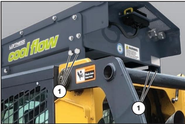
Remove the bolts (1) securing the rear legs to the mount (two bolts on each side of the oil cooler). Set the bolts aside.
