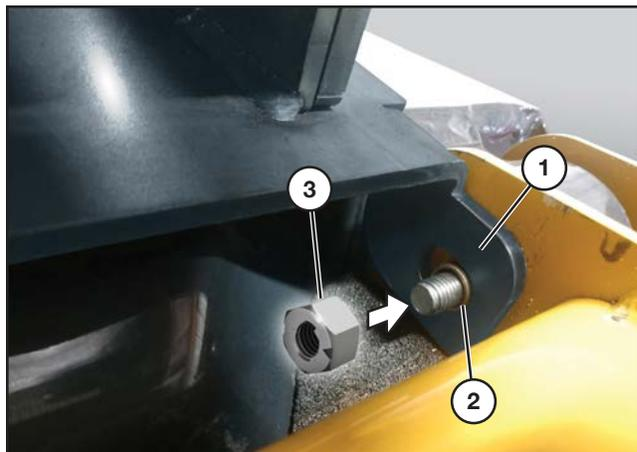
When setting the oil cooler cab kit down onto the cab, tip the back of the cab kit down to align the holes on the ears (1) of the cab mount to the bolts in the cab pivot.
