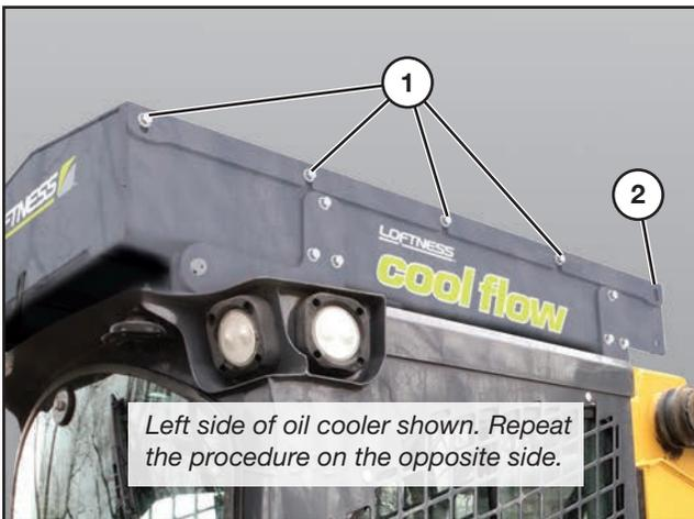
Loosen the remaining 8 bolts (1) (four on each side). Pivot the back end of the top cover up.
