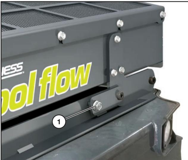
Remove the hex bolts (1) (one on each side of the oil cooler) that secure the lifting legs in the storage position.
